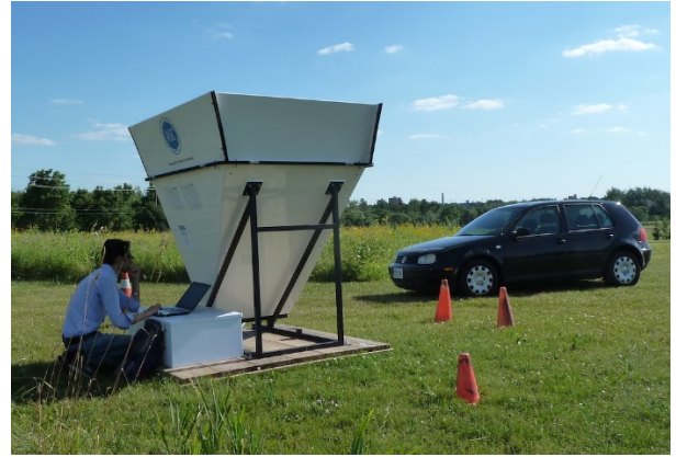
Figure 2. The Doppler miniSoDAR instrument operated in the rural area to measure the wind speed and direction profiles
